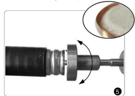
Use BXD07-6 to reshape the outer corrugation. Make sure to put the two shaping teeth inside the corrugation and then rotate until the outer corrugation is round enough with no dent or deformation and create visible clearance between outer corrugation and inner insulator.
