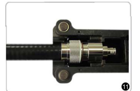
Put the connector into the compressing frame and make sure connector being sitted steadily.
