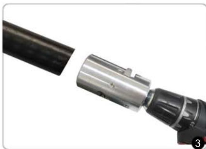
Insert the cable into the trimming tool. Select the low speed on the drill or 400~600 RPM on a variable speed drill. Trim the cable.
